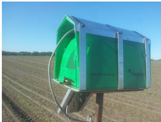
House constructed to make the trap stronger
